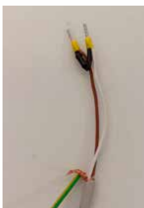
④ Green/yellow shield ground connection
