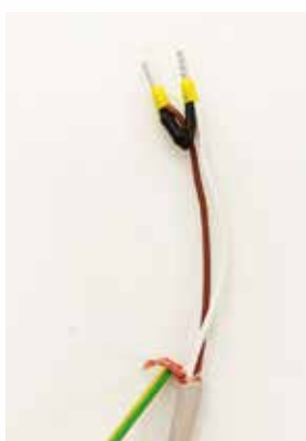
④ Green/yellow shield ground connection
