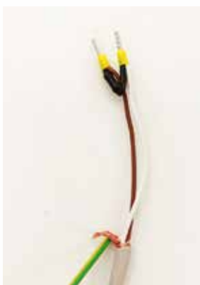
④ Green/yellow shield ground connection
